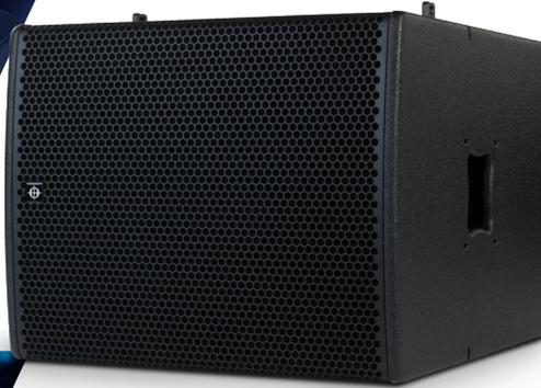
The N-SUB is a compact 15" high output subwoofer, weighing in at 28 kg. With high power handling of 1500 W, a maximum SPL of 139 dB (peak), this is a sub with guts - it reaches as low as 30 Hz.
