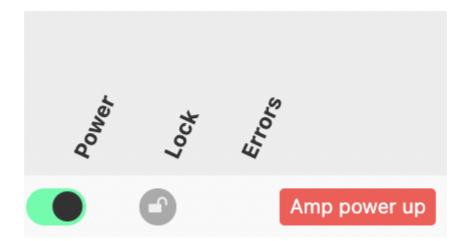
To place an amplifier in standby, or remove it from standby, using LINUS Control online, click the "Power" button in the AMPS page. This will toggle the amp between on and standby. The front panel switch works in combination with LINUS Control in a "Latest takes precedence" manner, which means LINUS Control can override a front panel switch and "wake up" an amplifier that's in standby with its front panel switch off.
