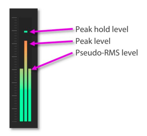
If the input meters are hitting the top (turning orange or red), and the loudspeakers are not in gain reduction, it would be best to assess the gain structure of the system to prevent overloading or overshooting the input stage, which can damage speakers. Attenuate the input signal and increase the system gain. We don't recommend that you clip the analogue inputs, it's not a sign of intellect!
