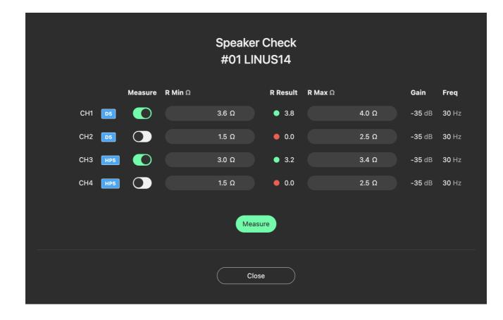
4. Connect amplifier channels with the loudspeaker and press "Measure". At this point you may hear the sine wave generator running (at -35dB / 30Hz) at a low level. The selected channels will be measured one by one, consecutively (measurement per channel takes roughly 3 seconds).
