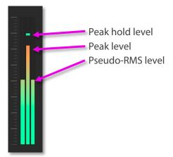
If the input meters are hitting the top (turning orange or red), and the loudspeakers are not in gain reduction, it would be wise to assess the gain structure of the system to prevent overloading or overshooting the input stage. Attenuate the input signal and increase the system gain. Don't be a silly billy and clip the analogue inputs, it's not a sign of intellect!
