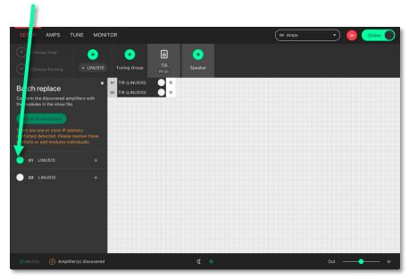
Select the destination amplifier in the workspace that you would like the replacement in the discovery list to take over from. This amplifier can either be Virtual, or Online. If it is an Online amplifier that is chosen as the destination, after the replacement is undertaken, this amplifier will itself then return to the discovery list.
