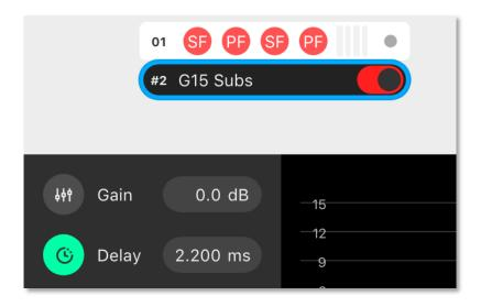
The Snapshot should now be stored on this amplifier, to enable offline recall from the Front Panel on site. Group Parameters (Gain / Delay / EQ etc.. can be adjusted from the Front Panel without use of the computer).
