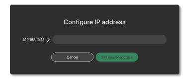
If the last octet of the new IP address is unchanged, the amplifier will show up on the workspace with the new IP. If not, it will show as offline on the workspace, and will show up as a newly discovered amplifier within the discovery list – it can then be replaced with the amplifier in the workspace using the standard method.
