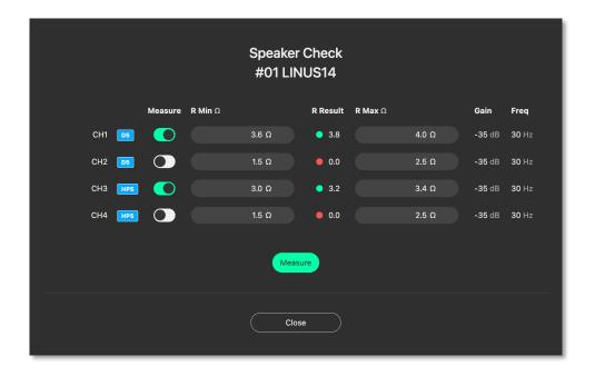
Note: The R Result values are dependent on many factors and may vary due to cable type and environmental conditions. Therefore, multiple measurements are recommended to the define proper R Min and R Max threshold values.
