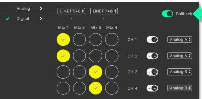
LiNET i/p 5 is routed to o/p CH 1 + 2 LiNET i/p 7 is routed to o/p CH 3 + 4 Fallback is ON.
