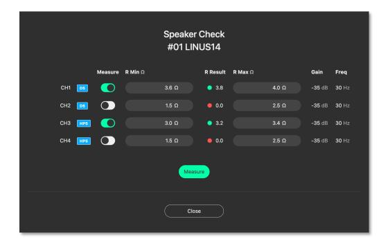
4. Connect amplifier channels with the loudspeaker and press "Measure". You might hear the sine wave generator running (at -35dB / 30Hz) at low level. The selected channels will be measured one by one, consecutively (measurement per channel takes ca. 3 seconds).
