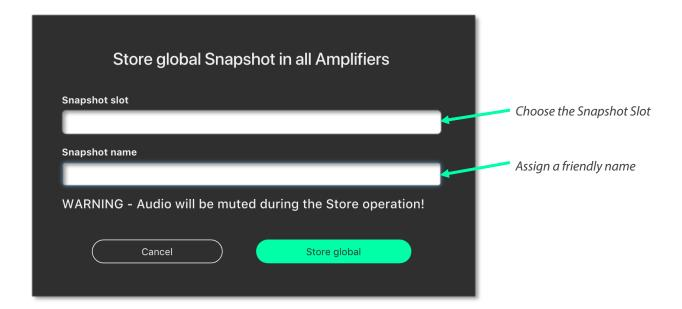
Note: The software will report [mixed snapshots] in the 'Snapshot slot' list if snapshots with different names are stored in the same slot in multiple amplifiers.
