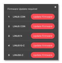
Note – If after pressing the 'Update Firmware' button, it reappears again after a short period of time, power cycle the amplifier. Once the 'Update Firmware' button is pressed, the amplifiers will disappear out of the discovery list. Please wait at least 30 seconds for the amplifiers to show up again in the discovery list.
