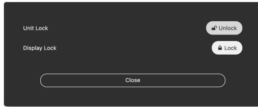
To unlock the amplifier, press this (Unlock) button, then enter the password into the dialog that is presented:
