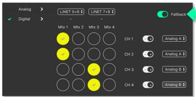
LiNET i/p 5 is routed to o/p CH 1+2LiNET i/p 7 is routed to o/p CH 3+4Fallback is ON. Analog A is the Fallback source for CH 1+2
