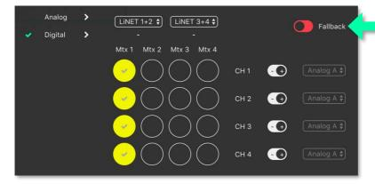
LiNET i/p 1 is routed to all o/p Chans. Fallback is OFF All o/p's are in Polarity
