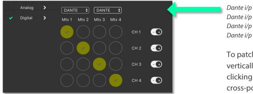
Dante i/p 1 is routed to o/p CH 1 Dante i/p 2 is routed to o/p CH 2 Dante i/p 3 is routed to o/p CH 3 Dante i/p 4 is routed to o/p CH 4
