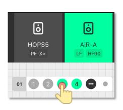
When the loudspeaker is in 'ASSIGN' mode, the channels can be selected that the loudspeaker should be assigned to.
