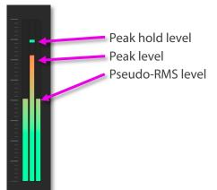
If the input meters are hitting the top (turning orange or red), and the loudspeakers are not in gain reduction, it would be wise to assess the gain structure of the system to prevent overloading or overshooting the input stage. Attenuate the input signal and increase the system gain. Don't be a silly billy and clip the analog inputs, it's not a sign of intellect!
