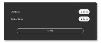
Pressing the (Lock) button to the right of the Display Lock text will toggle the display lock state
