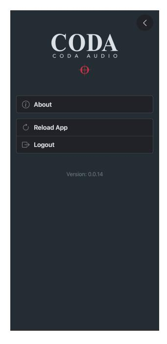
The button (three horizontal lines) in the top left of the App's user interface opens the App menu. If the App ever gets disconnected from the amplifier for whatever reason, please click the "Reload App" button. This will reconnect to the amplifier and refresh the current state.
