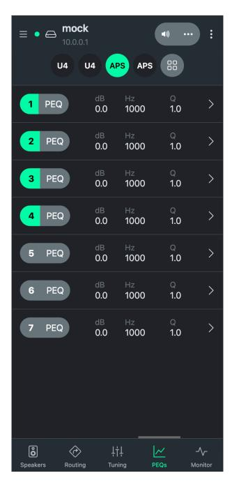
The PEQs Tab offers 7 additional parametric equalisers for each output channel. A PEQ is enabled if its number is highlighted in green. The filter type can be set to either Bell, High-Shelf or Low-Shelf. A PEQ can be adjusted by clicking its row in the PEQ list.
