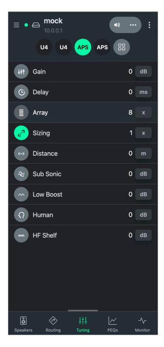
In the Tuning Tab, you will find the same Tuning Tools as in LINUS Control. Click on the abbreviated loudspeaker name at the top of the Tuning Tab to select that channel for tuning. To apply the same tuning parameters to multiple channels, channels can be grouped at the top of the page.
