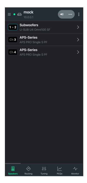
In the Speakers Tab, you can load speaker presets without connecting to LINUS Control. Clicking a channel opens the Preset list, containing all speaker presets that are currently supported for LINUS6.4. At the top of the Preset list, you can switch between Single-Ended ("Normal") and Bridge Presets. Bridged channel pairs are displayed as one channel in the Speakers Tab (e.g.: "1+2").
