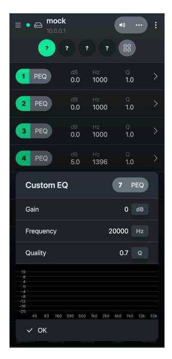
This will open a windows with parameters for filter type, gain, cutoff frequency and bandwidth. The Grouping logic in the PEQs Tab works the same as, and is mirrored in the Tuning Tab.
