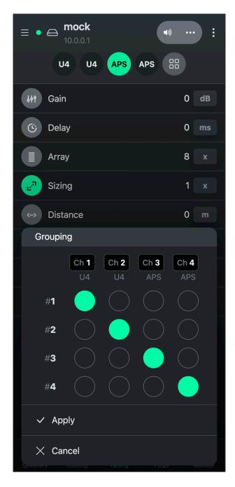
Here you can link multiple amplifier channels (columns) to one virtual Tuning Group (rows). The same Grouping logic applies to the PEQs Tab.
