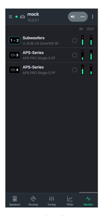
The Monitor Tab shows Input and Output signal levels of the individual amplifier channels. Bridged channel pairs are displayed as one output ("1+2" for example). Click a channels to open a more detailed meter view.
