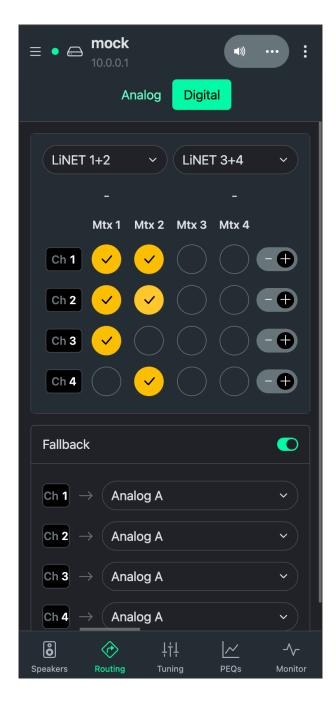
The Routing Tab offers the same input routing options that can be found in LINUS Control. At the top, you can switch between Analog and Digital inputs. To the right of each line in the Routing Matrix, there is a polarity invert switch for that amplifier output. If LiNET is selected as input signal type, the Analog Fallback Routing list appears below the Routing Matrix.
