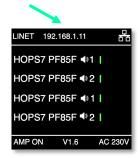
All devices should have an individual IP address configured (within a given range).
