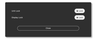
Pressing the (Lock) button to the right of the Display Lock text will toggle the display lock state of the relevant amplifier. An 'L' or 'Padlock' icon will be displayed on the amplifier LCD.
