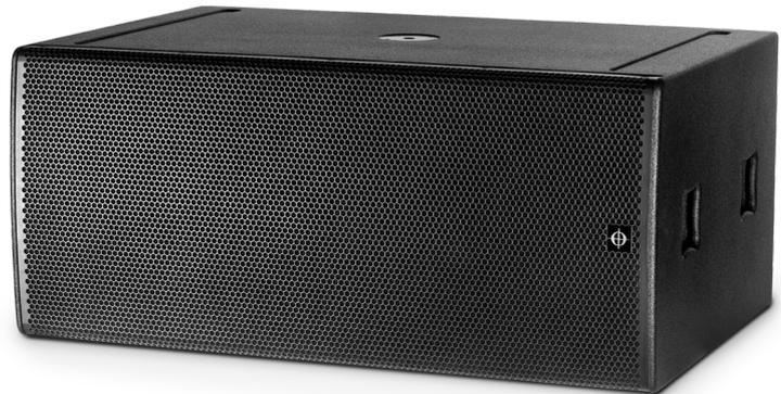
The U4-Sub is equipped with twin extremely long excursion 18" ultra low distortion woofers. The strong motor delivers extreme high magnetic flux for increased efficiency.
