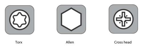
Image 8: Three types of fixing heads used
