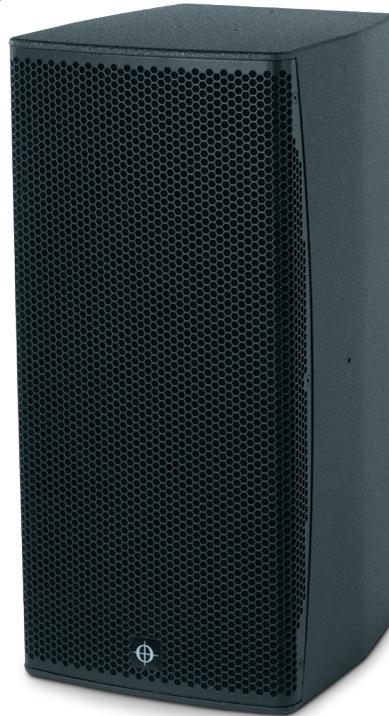
The CODA HOPS12i is an extremely high output 3-way installation point source featuring dual 12" neodymium ultra low distortion cone drivers and a 1.4" mid/high driver in a compact enclosure. The loudspeaker is available with different dispersions providing variable directivity to many installation applications - for instance, dance clubs, houses of worship, sport venues, theatres and corporate events.
